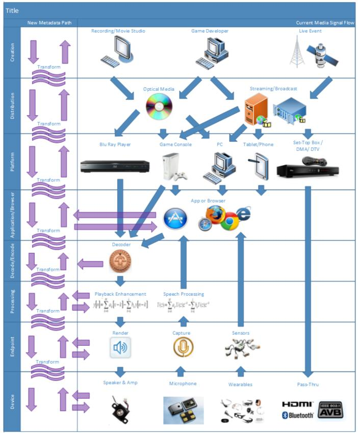
This diagram shows in blue the current signal flow for many different combinations of devices. The violet arrows show the recommended path for metadata. The metadata transforms occur as the metadata is passed from stage to stage, adding or removing metadata along the way.
